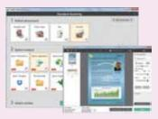
The TOP screen is laid out panelstyle with large icons, allowing more intuitive operation. The items on the setup screen have also been scaled down to give a simple design. Two scanning methods are available to satisfy a variety of needs including adhoc and daily scanning. As well as "Standard Scanning" where scanning mode and output mode can be separately configured, there is
